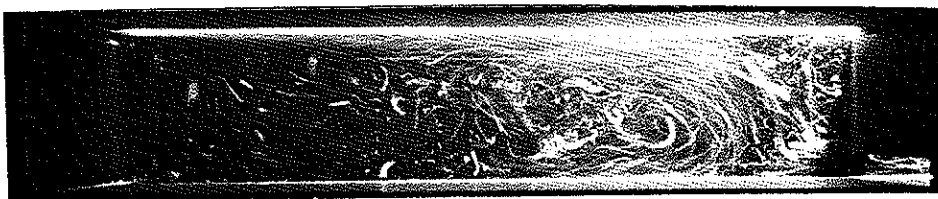
Fig. 2.4.3-2. Unsteady flow in model with length L/H = 5.0 and big width. h/H = 0.056 , w/W = 1.0 , W/H = 4.7 , u/H = 0.16 and Re = 7000 .
