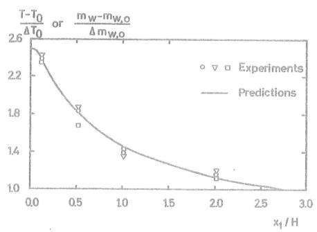
FIG. 1 Comparison between predicted and measured temperature or mass distribution. h/H = 0.056, L/H = 3.0 and Re= 7100.
