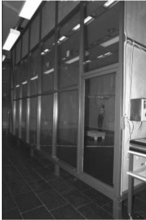
Figure 3.5. Photo of the full-scale test room with a floor area of 48 \text{ m}^2 and a height of 4 m in the present set-up. On the photo the double glazing in one of the walls is seen, applied to facilitate smoke visualisation.
