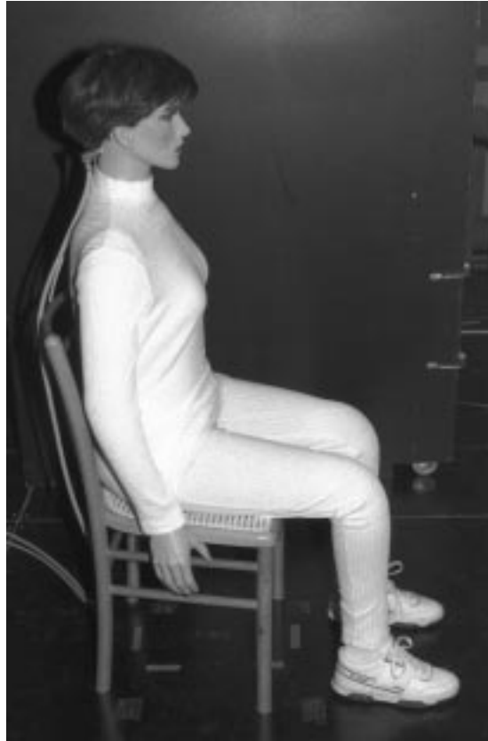
Figure 2.7. Breathing Thermal Manikin used to measure the personal exposure. The manikin is separated in 16 individual parts of the body, each with the same surface temperature and heat output as people in thermal comfort. The manikin has an artificial lung to simulate breathing. Height = 1.7 m, A_{Du} = 1.5 \text{ m}^2 , I_{cl} = 0.8 clo.
