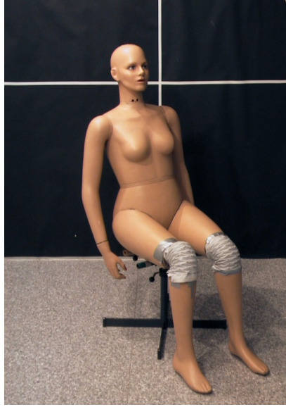
Figure 8.2: Picture of the breathing thermal manikin used in the experiments by Holsøe [47].
