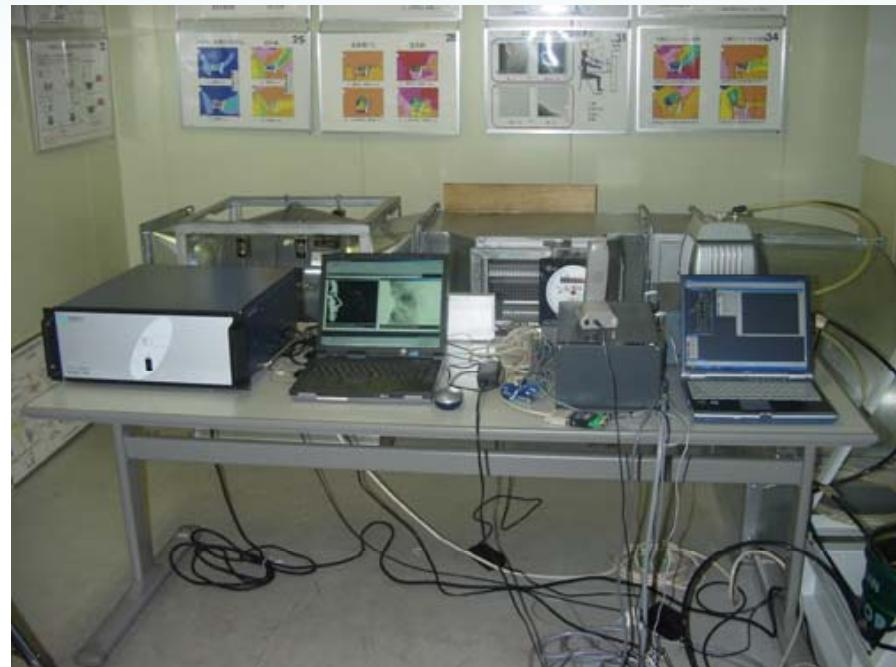
Equipments of PIV and controller of thermal manikin
