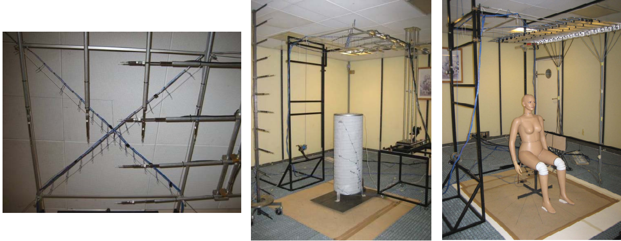
Figure 2. Basic position of sensors and set up for testing the cylinder and the rectangular box (left and middle), and set up for testing the dummy and the thermal manikin (right).
