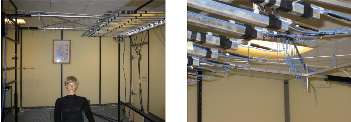
Figure 1. Position of sensors at the level of 0.7 m above the manikin head.
