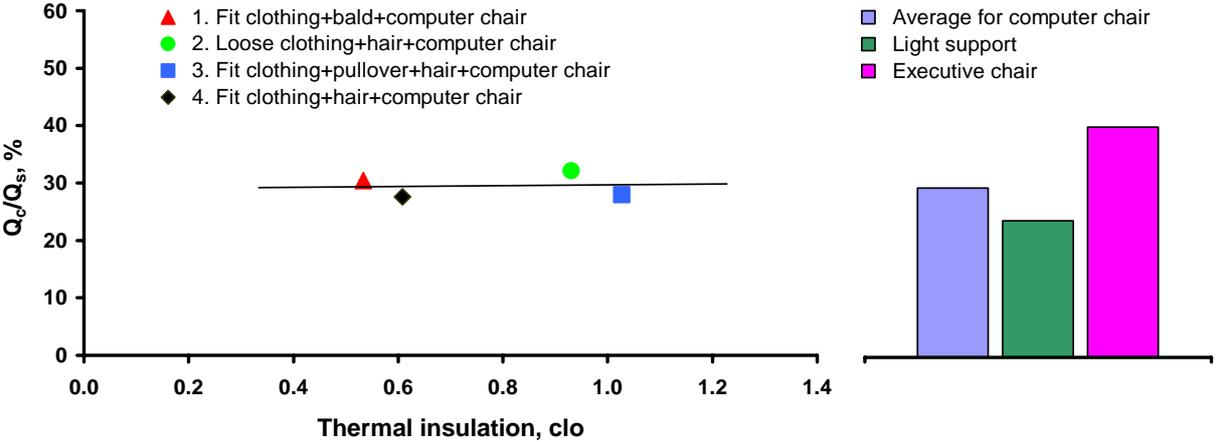
Figure 4. Ratio of convective heat to power supplied to the sitting manikin as function of clothing and chair insulation.
