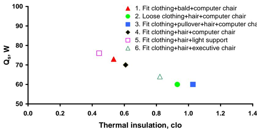
Figure 3. Power supplied to the manikin as function of clothing and chair insulation.
