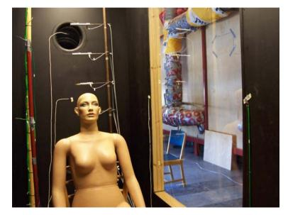
The flow field situation was made as identical to the earlier benchmarks with the intention that data will be interchangeable and comparable between the two tests.
