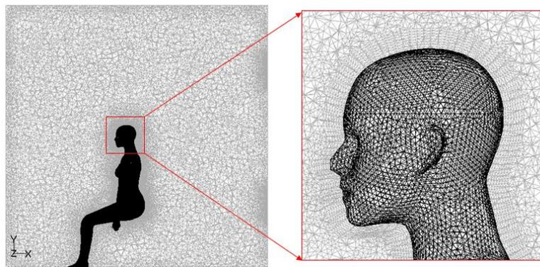
Figure 3. A Cross-Section of the CFD Volume Mesh (gray) and Surface Mesh of the Manikin (black)
