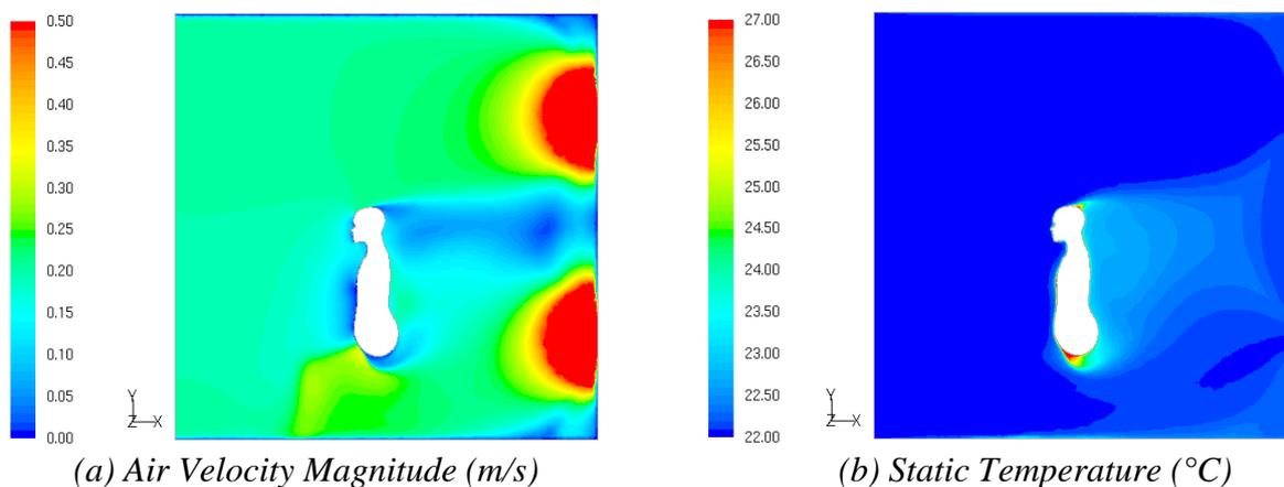
Figure 5. Contours of Air Velocity and Temperature on the Vertical Mid Plane at  $Z = 0.6$  m
