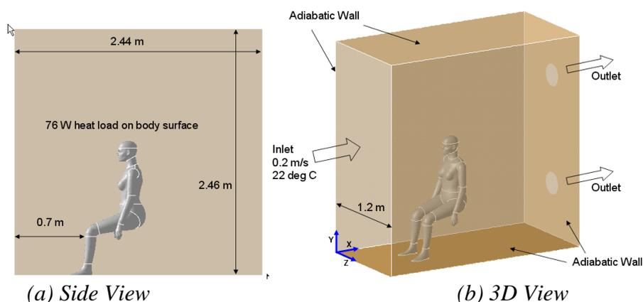
Figure 2. CFD Model of the Test Room with the Simulated Manikin inside
