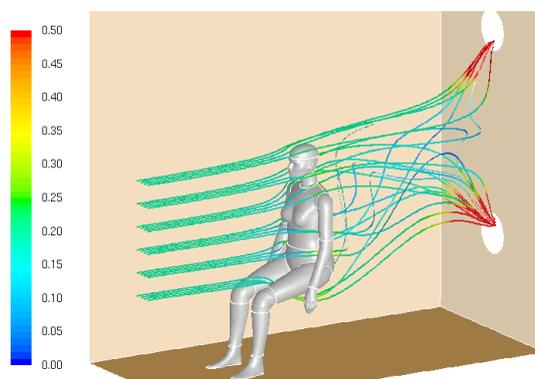
Figure 4. Streamlines inside the Test Room and Around the Simulated Manikin (Colored by velocity magnitude with a unit of m/s)
